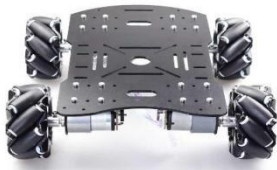
Gambar 1: Mekanik robot omnidirectional
